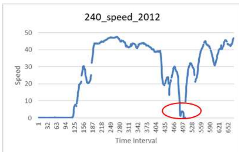
Figure 99 Vehicle speed profile and roadworks detection 1
