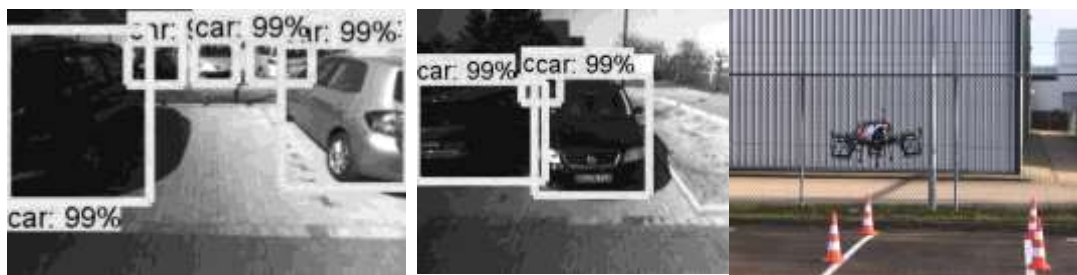
Figure 7 MAV parking spot occupancy detection (Left: occupied, middle: free, right: MAV in flight)
