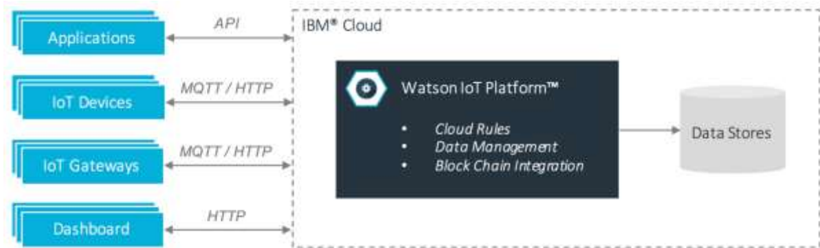
Figure 4. Architecture of the Watson IoT Platform™
