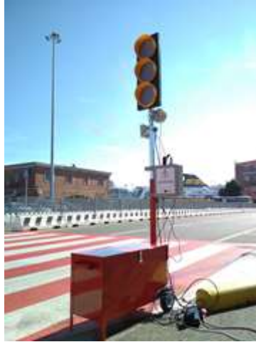
Figure 20. Picture of the smart traffic light with RSU and camera for pedestrian detection
