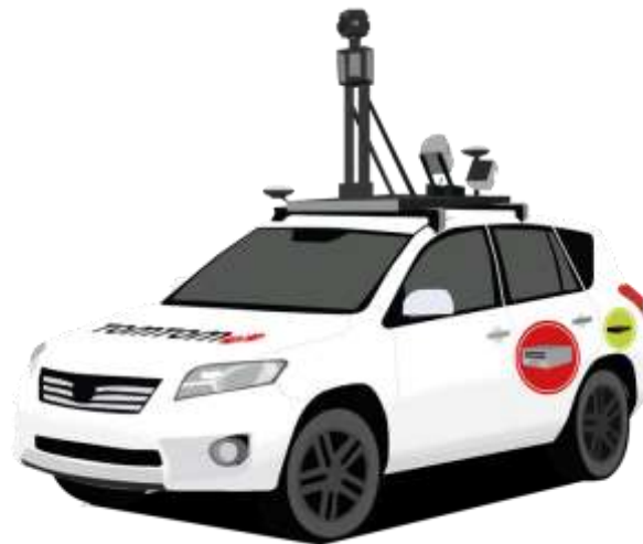
Figure 21–TomTom survey vehicle used for adding automotive grade sensors for localization
