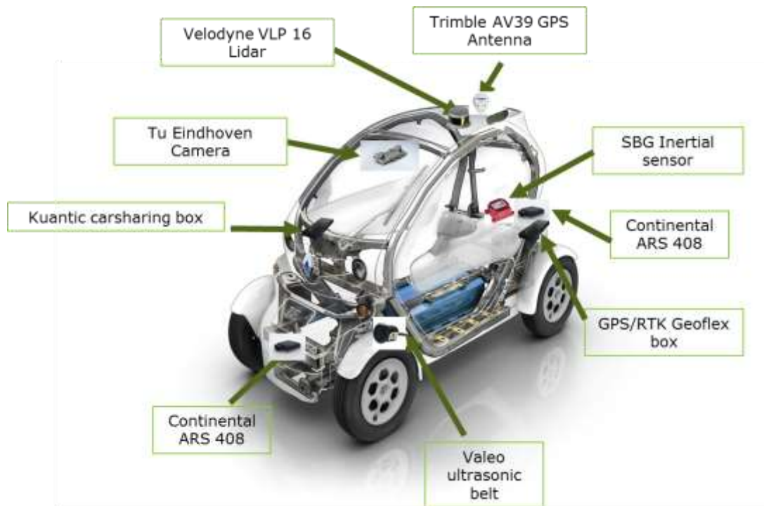
Figure 8 – Overview of VEDECOM prototype sensors
