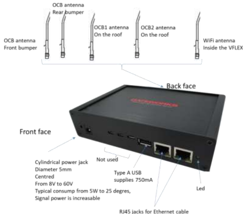
Figure 12 – Gateworks Ventana SBC inside its enclosure
