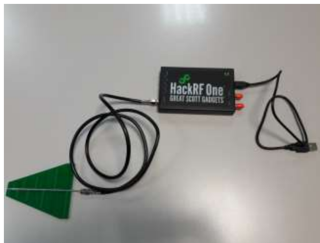
Figure 2: The HackRF One SDR with the logarithmic antenna used in this context
