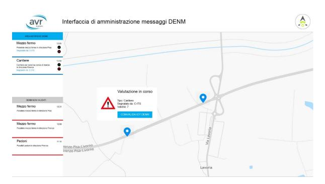
The DENM interface will be used by AVR TCC to geolocalize and validate events exchanged between the devices and the cloud platform
