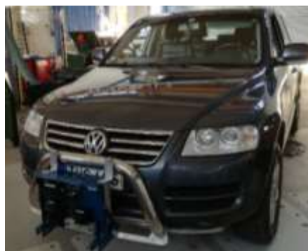
Figure 6 – Sensor kit installed in VTT's pilot vehicle Martti
