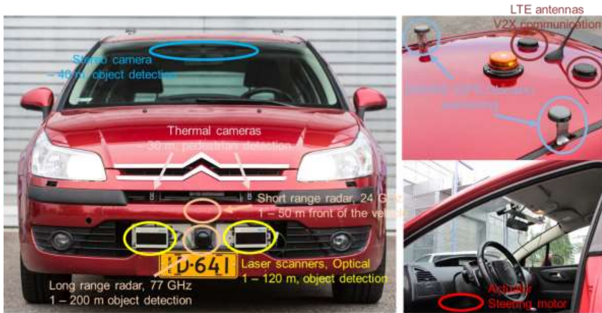
Figure 5 – Sensors installed in the Finnish automated vehicle prototype
