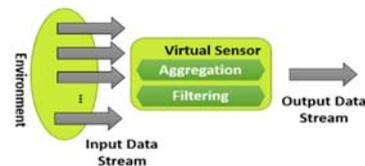
Figure 3: "Virtual Sensor" concept.
