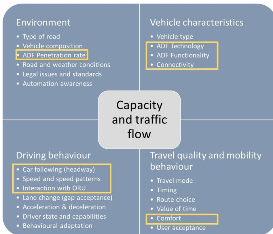
**Figure 3 - Factors of automated driving affecting capacity and traffic flow (The areas where IoT is expected to play an important role are highlighted with yellow borders).**
