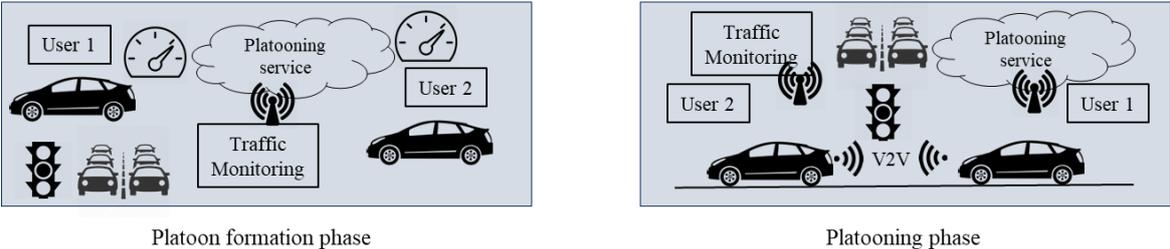
Figure 3 – Schematic representation of the platoon formation and platooning phases.
