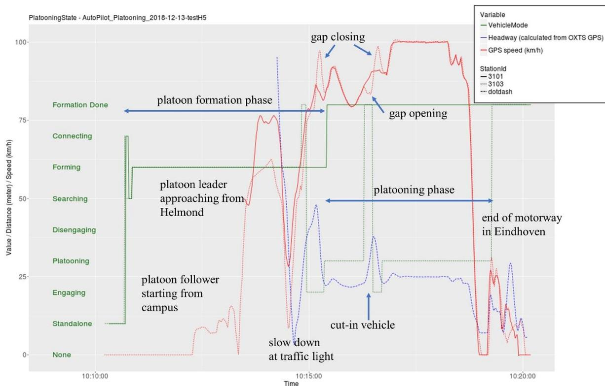
**Figure 5: Analysis of a platooning run, showing states and speeds of the vehicles and headway.**
