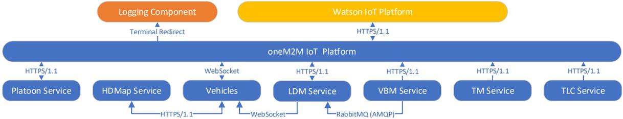
Figure 2 - Logical overview of IoT components used in the platooning use case.
