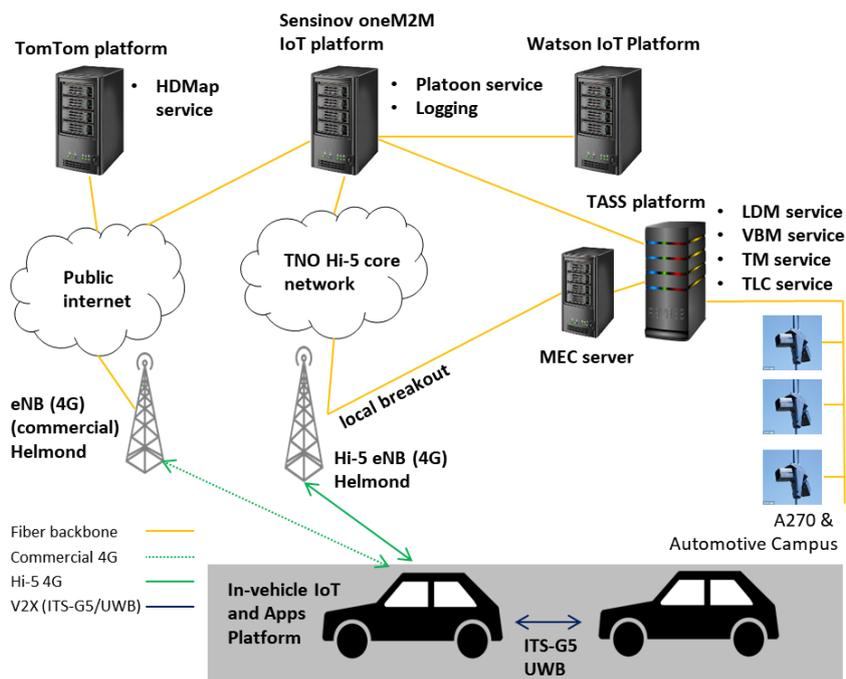
**Figure 1 - Pilot site architecture overview for the platooning use case.**
