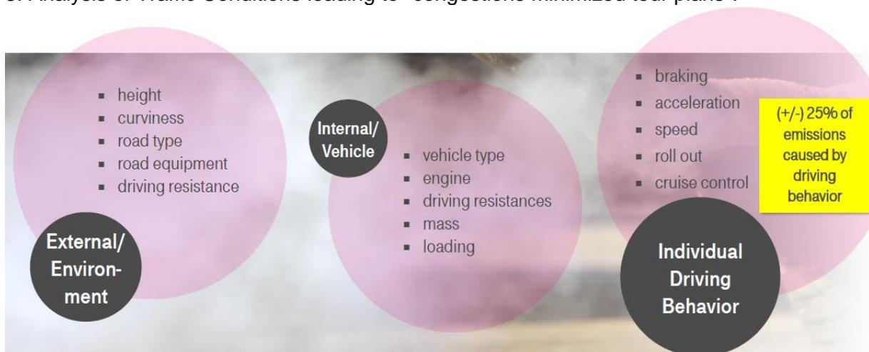
**Figure 1: Influence factors for NO<sub>2</sub> emissions in vehicle based road traffic**
