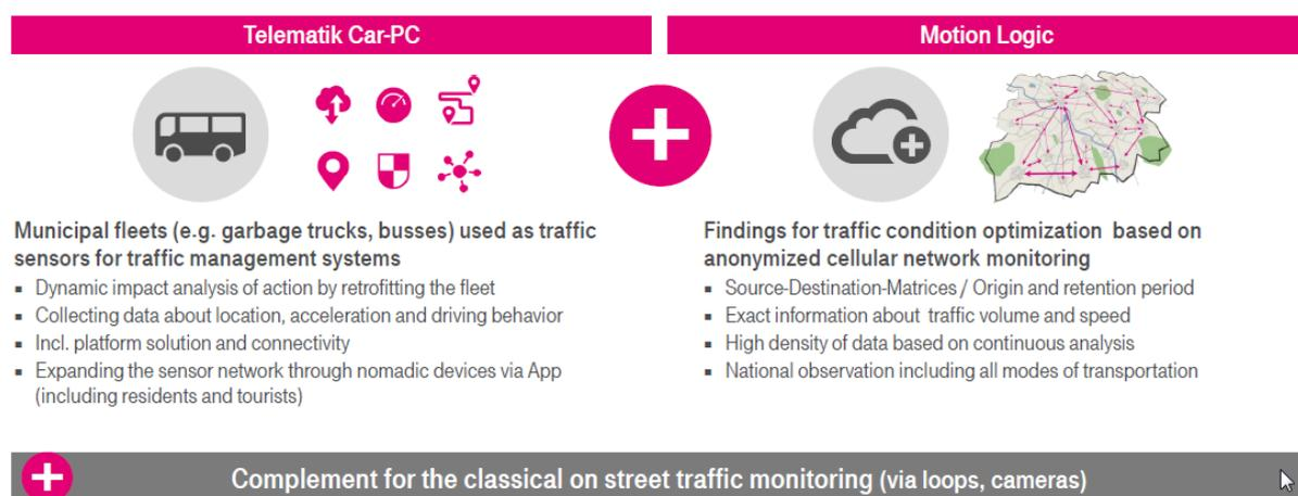
**Figure 3 Extended data collection strategies based on multi-source integration of fixed and mobile data from Floating Cars with telematics devices as well as anonymized cellular speed profiles from telecommunication networks**
