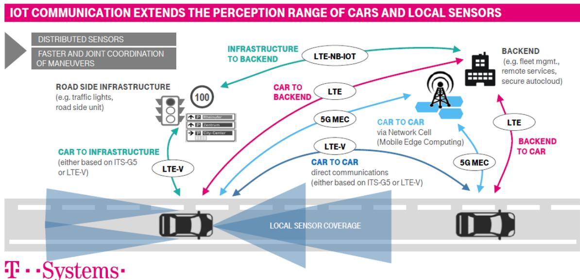
Figure 5 Schematic overview of the different data exchange objects relevant for IOT based Automated Driving service deployment
